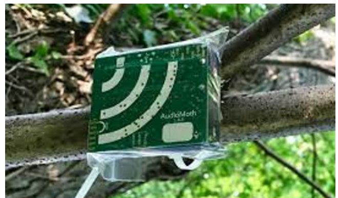
AudioMoth low-cost, open-source acoustic sensor (© Open Acoustic Devices)
