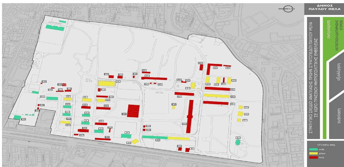
Figure 8: Building stock: 24.292 m<sup>2</sup> built surface. Green-16% (4.115 m<sup>2</sup>) in good condition, Yellow-26% (6.531 m<sup>2</sup>) in moderate condition and Red-58% (13.646 m<sup>2</sup>) in bad condition
