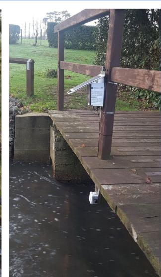
Our //Smart:River web connected, low cost, DIY sensors are monitoring the contribution of leaky dams, retention ponds and conservation agriculture to flood mitigation at sites throughout England
