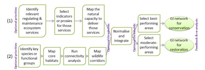
Fig. 2. Methodological workflow for the identification and mapping of GI networks. Modified from EEA (2014) and Liquete et al. (2014).
